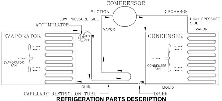
The Compressor, Condenser, Drier, Capillary Tube, Evaporator, and Accumulator are part of a sealed system (refer to figure 16). These items are not available separately. For the part number of the sealed refrigeration system refer to the common parts section of the manual.
