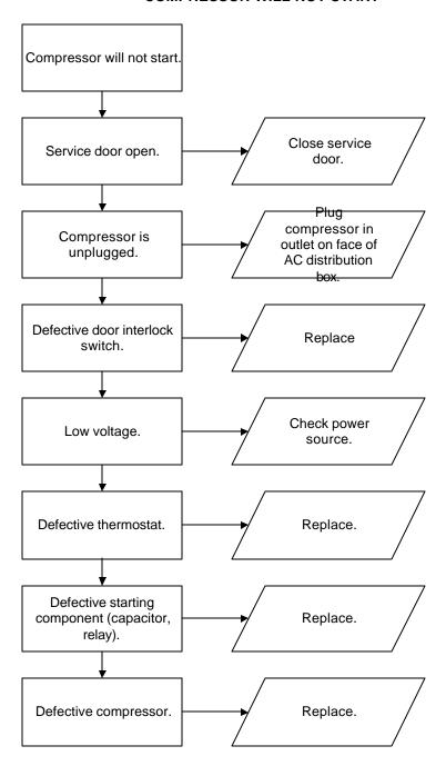
Troubleshooting Tip: Use a short 15 Amp extension cord and plug the compressor directly into the wall outlet. This will bypass the AC distribution box. Note: For Testing Purposes Only.
